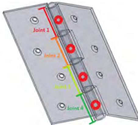
When viewing pin connector results, in the Result Force PropertyManager, click a table cell under **Connector Force** to highlight the location of the selected pin joint. A callout lists the pin forces at the selected joint. The directions of the pin resultant forces with respect to the pin's local coordinate system are also displayed: shear force resultant, axial force resultant, bending moment resultant, and torque resultant.
