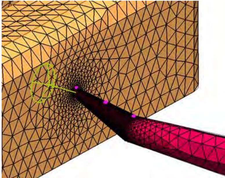
When you have both solid and shell mesh in a study, the inactive mesh node is unavailable. The inactive mesh node is highlighted in gray.
