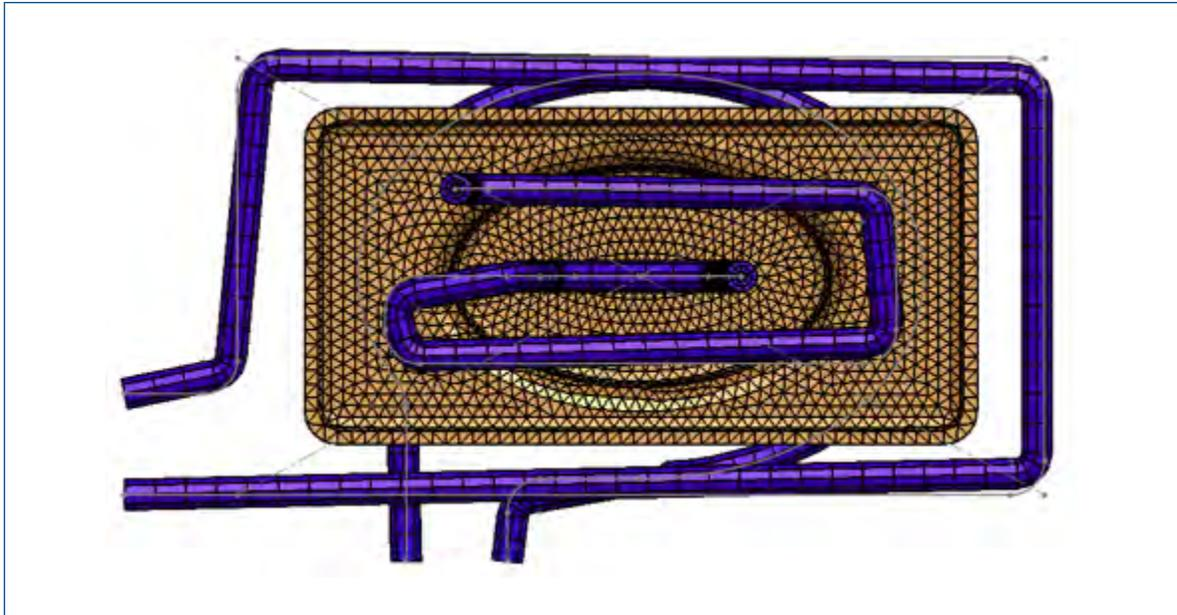
Meshed Cooling Channel (SOLIDWORKS Plastics 2018)
