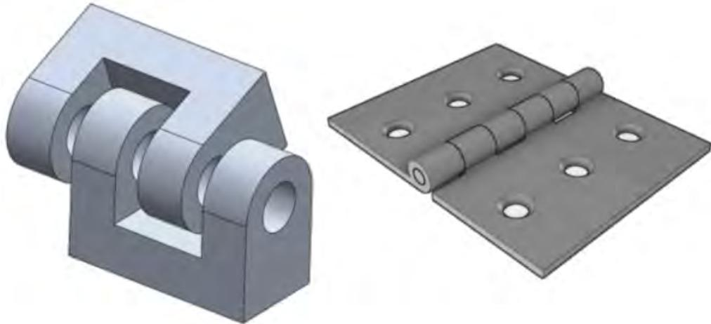
The solver calculates the pin connector forces at two pin joints per pin segment (a pin segment attaches to two cylindrical faces.) The safety factor for each pin connector is calculated based on the least FOS at the pin joints for the selected pin connector. The total axial and rotational stiffness you define for a pin connector is distributed according to each pin segment's geometric characteristics such as: cross sectional area, length, and polar moment of inertia.
