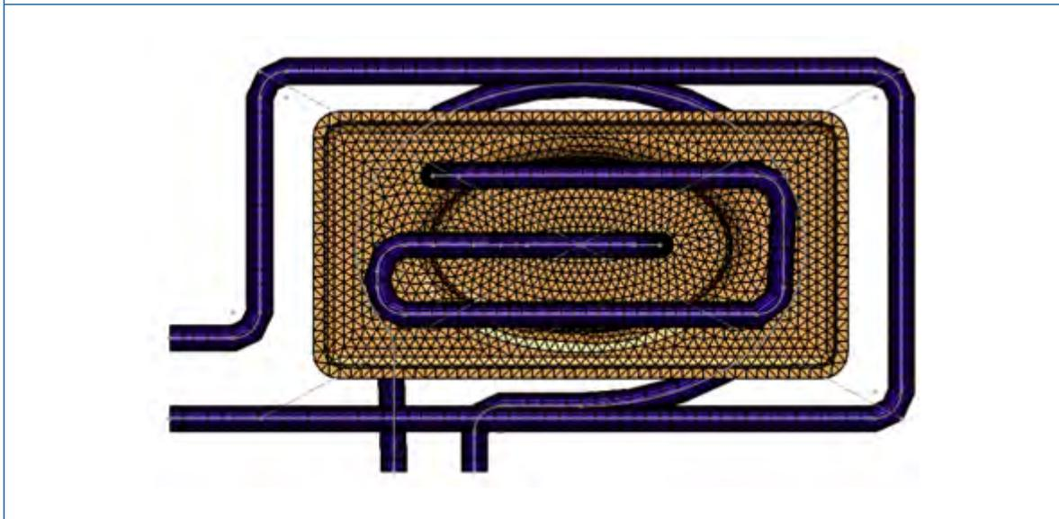
Enhanced mesh for Cooling Channel (SOLIDWORKS Plastics 2019)
