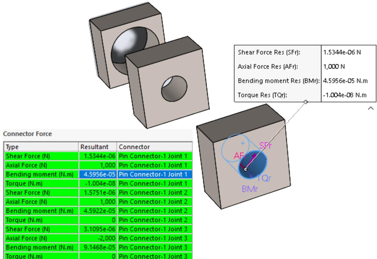
Click **List X,Y,Z components** to list the X, Y, and Z components of the pin forces with respect to the global coordinate system.
