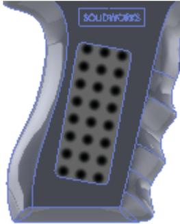
Try to fit the textural appearance so all the circles are within the handle boundary and do not intersect the surrounding edge. You do this to create a closed, watertight model that you can 3D print.
