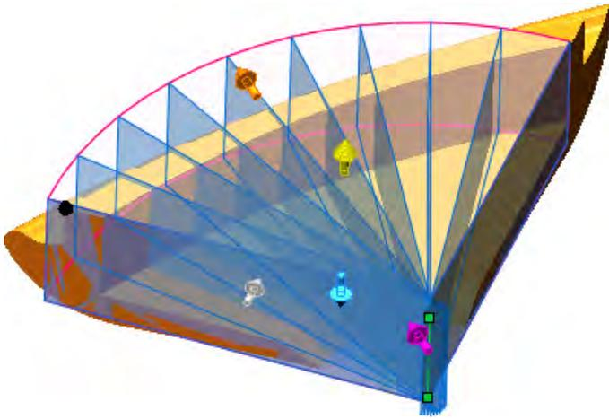
5. Drag the orange handle to enclose the whole model with the bounding box.
